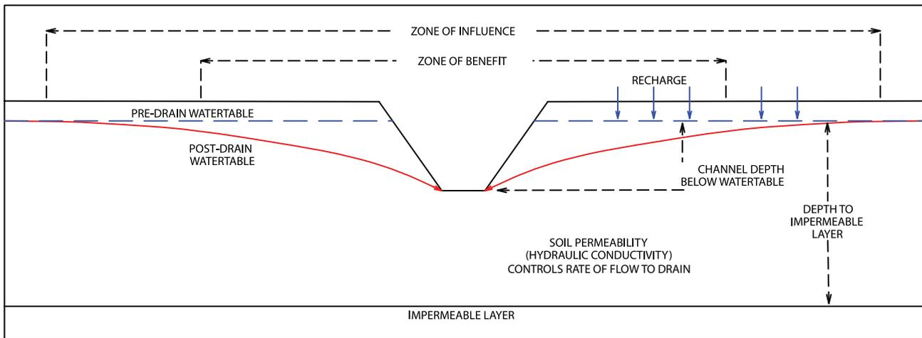
Figure 3 The main variables affecting the performance of a groundwater drain
