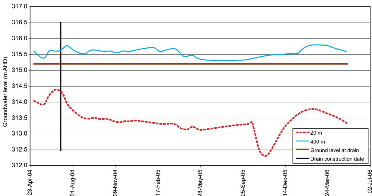
Figure 4 Time series groundwater level responses to drainage in bore transect 3
