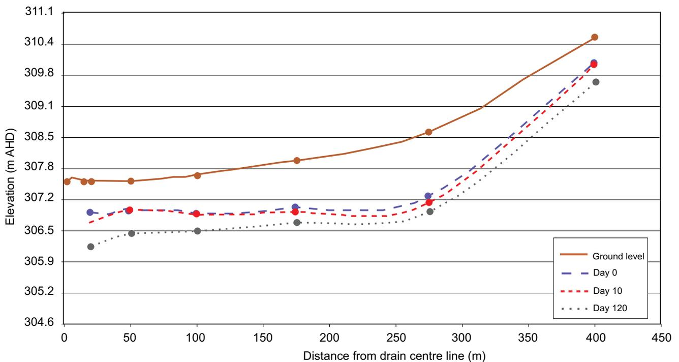
Figure 5 The average groundwater profiles for all transect bores in the Pithara drainage site for days 0, 10, and 120
