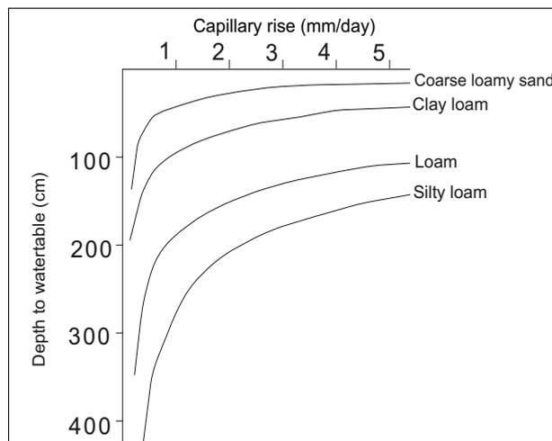
Figure 2 Rates of evaporative loss from different soils with watertables at various depths
