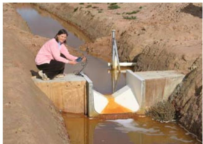
Sylvia Tetlow measuring the salinity and pH of the water at the downstream gauging station at Pithara. The orange staining on the flume and drain is due mainly to precipitation of iron from the groundwater.
