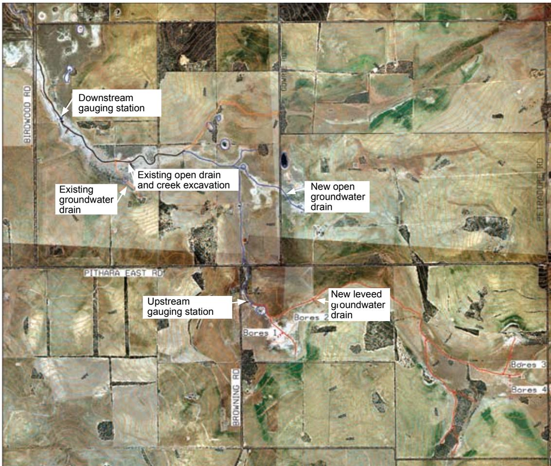
Figure 1 Aerial photograph and illustration of the drain alignment and main features of the Pithara drainage site
