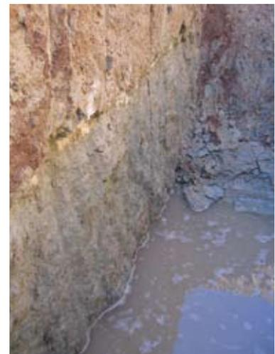
Soil profile of backhoe pit showing groundwater
