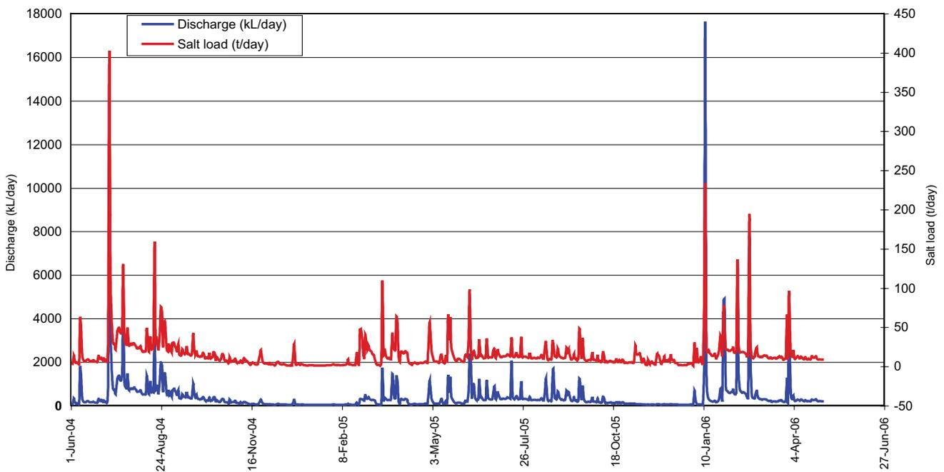
Figure 7 Discharge and salt load for the downstream gauging station
