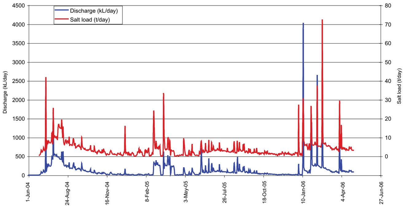
Figure 6 Discharge and salt load for the upstream gauging station
