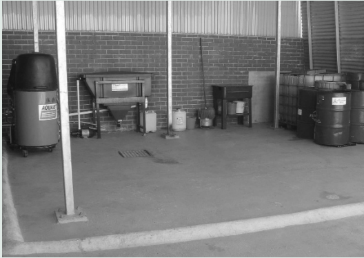
Figure 1. Green Stamp automotive premises, Balcatta. Under-cover, bunded wash-down area, with parts washer, wastewater treatment equipment and drums for recyclable materials. (Photograph: Department of Environment.)
