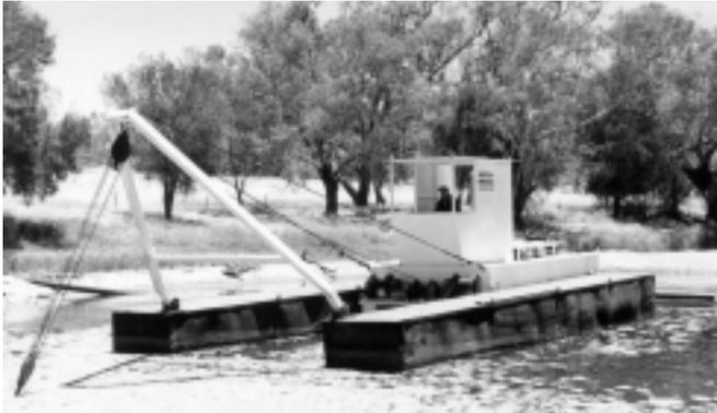
*Photos showing the accumulation of sediment in Burlong Pool near Northam. The dredge is used to excavate sand with an estimated 10,000m<sup>3</sup> being removed from Burlong Pool annually.*
