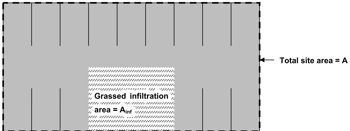
Figure 4. Example definition of a catchment area where the infiltration surface is located within the defined site area.
