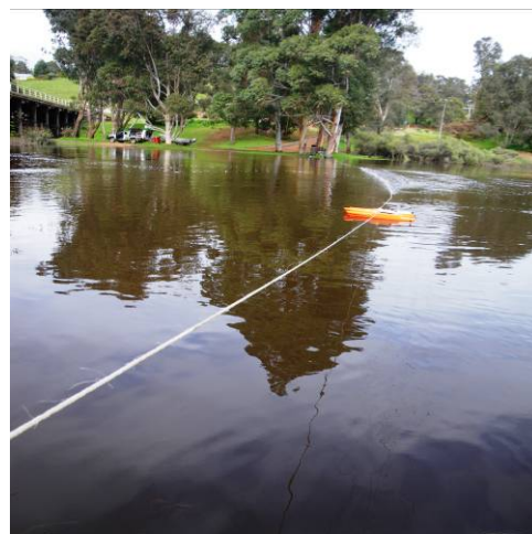
Measuring river flows (volume) at Bridgetown
