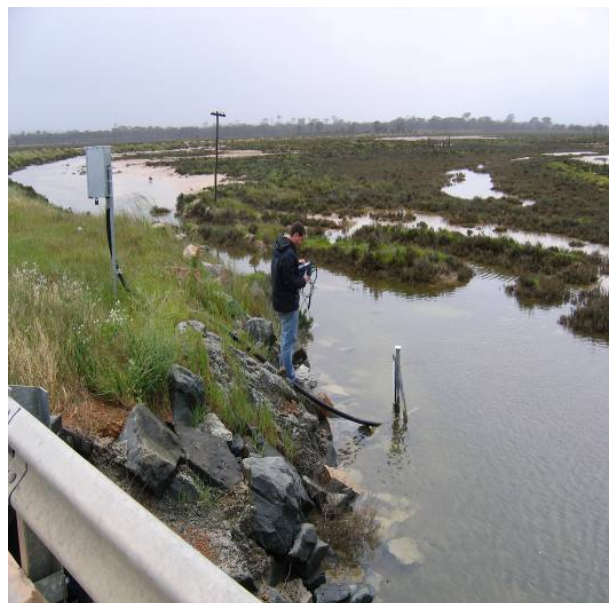
Continuous conductivity meter in the Dongolocking Creek
